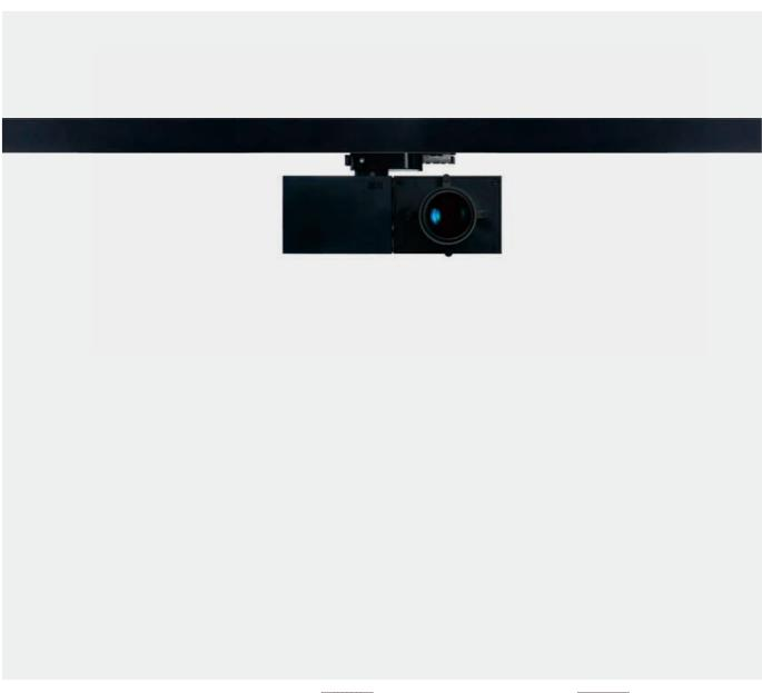
Dux A3 fine art projector is designed for precise lighting of museum exhibition space within 3 meters and cultural relics in exhibition cabinet. With M3's delicate size and precise high transparency optical lens, weighing only 550g, Dux A3 has 12W wattage and beam angles of 12°, 19° and 36°. It can provide customized precise lighting for exbihits in low-space display space of museums and galleries, such as crowns, jades, bronzes, coins, small paintings and calligraphy, etc.
