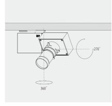
Vertically 270° rotation, lighting both downward and upward. Dux A3 continues the flexible lighting of the Tracron track lights. The whole lamp can be rotated historical details to be
